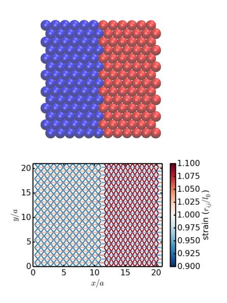
Cost of deforming domain to fit in box:  $E = Y(L - L_0)^2$
